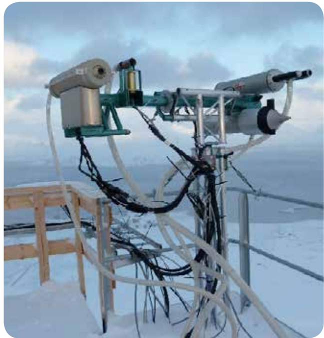
Figure 3 : Instruments for the characterization of cloud properties installed on the terrace at the Zeppelin Station at an altitude of ~480 m.
