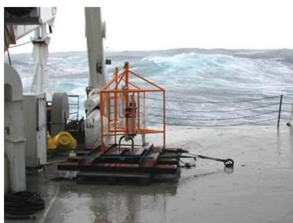
Figure 5: Left: Autonomous tide gauge station on the deck of the Marion-Dufresne ship waiting to be moored. Right: Raising the continental shelf tide gauge station on board the Marion-Dufresne ship.
