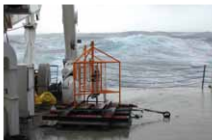
Figure 5: Autonomous tide gauge station waiting to be moored, installed on board the Marion Dufresne vessel. © LEGOS/OMP, INSU-CNRS.
