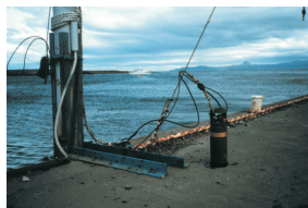
Figure 2 : Pressure and Temperature Aanderaa sensor in Kerguelen
