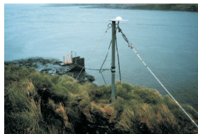
Figure 3 : The Argos antenna and the tide gauge station below (Crozet)
