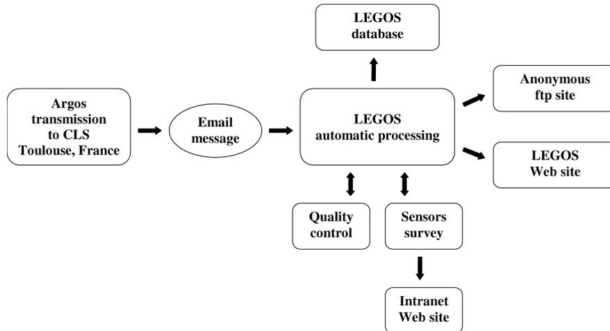
**Figure 3: Automatic acquisition/quality control/fast delivery software**
