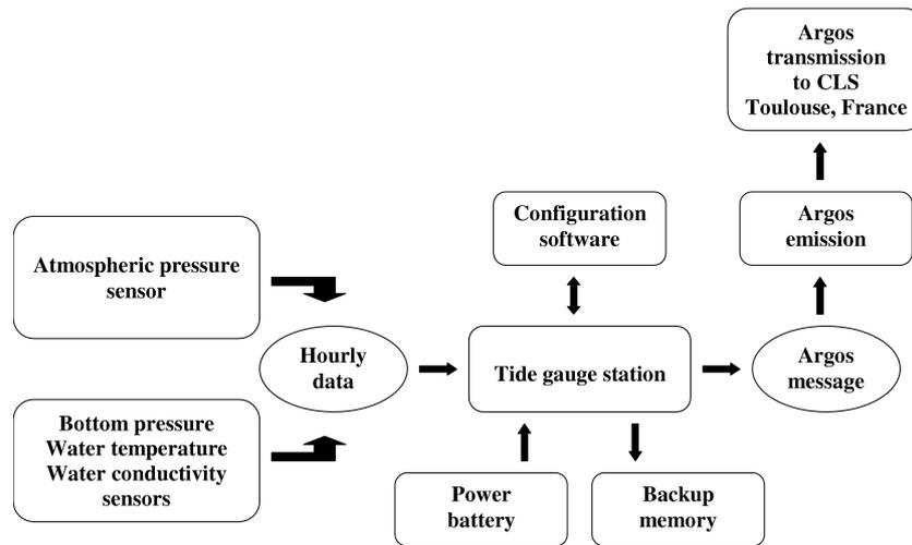
**Figure 2: Automatic real time acquisition and transmission of data**
