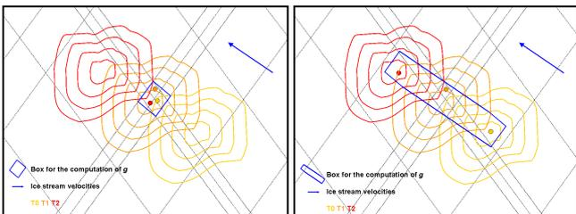
Left: we don't take into account ice stream effects. The size of boxes for the geographical function computation only considers altimeter positioning errors. Right: we consider ice flow. The boxes are extended in the flow direction with a  $V_{ice} \times time\ elapsed\ distance$ .
