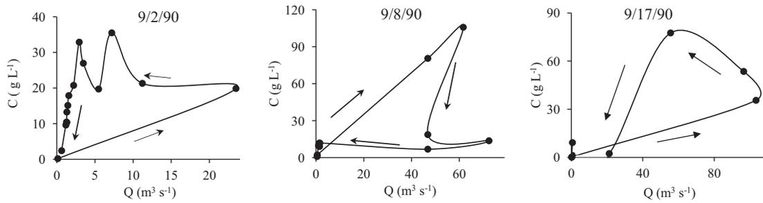
Fig. 5. Influence of timing of flood events on sediment yield: the example of three floods in September 1990.
