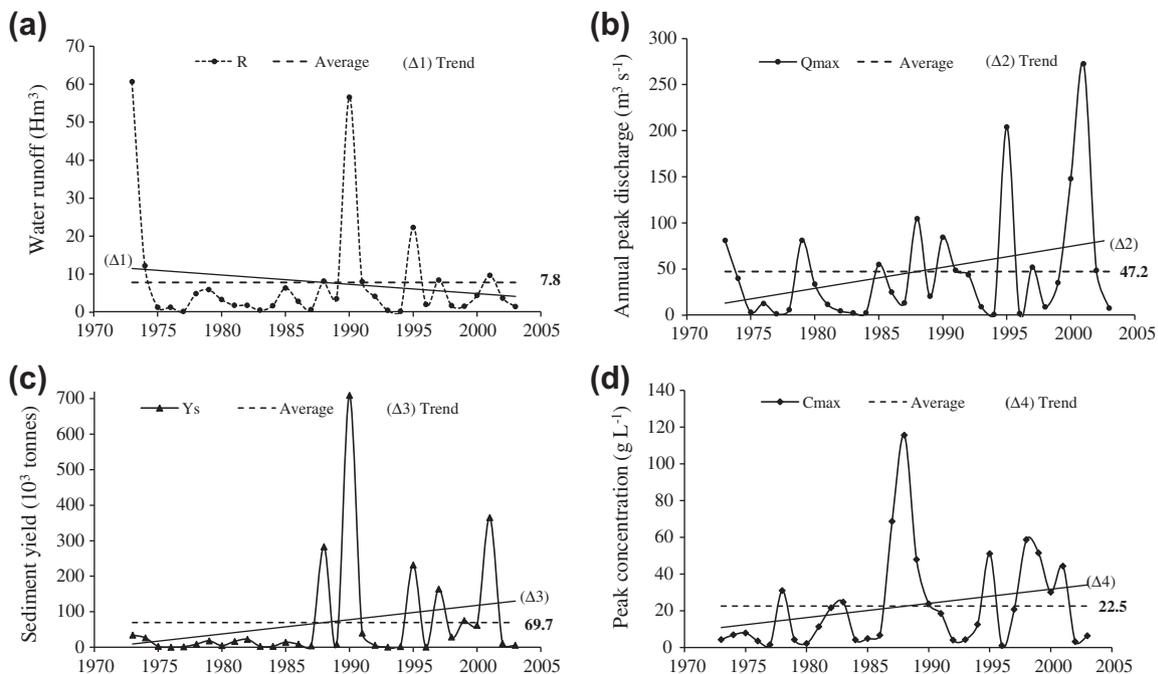
Fig. 3. Trends of annual peak floods for the period September 1973–August 2004. (a) Runoff of the annual maximum flood flows, per year, and (b) the corresponding peak discharge. (c) Sediment yield of the annual flood of maximum sediment delivery, and (d) the corresponding sediment concentration peak.
