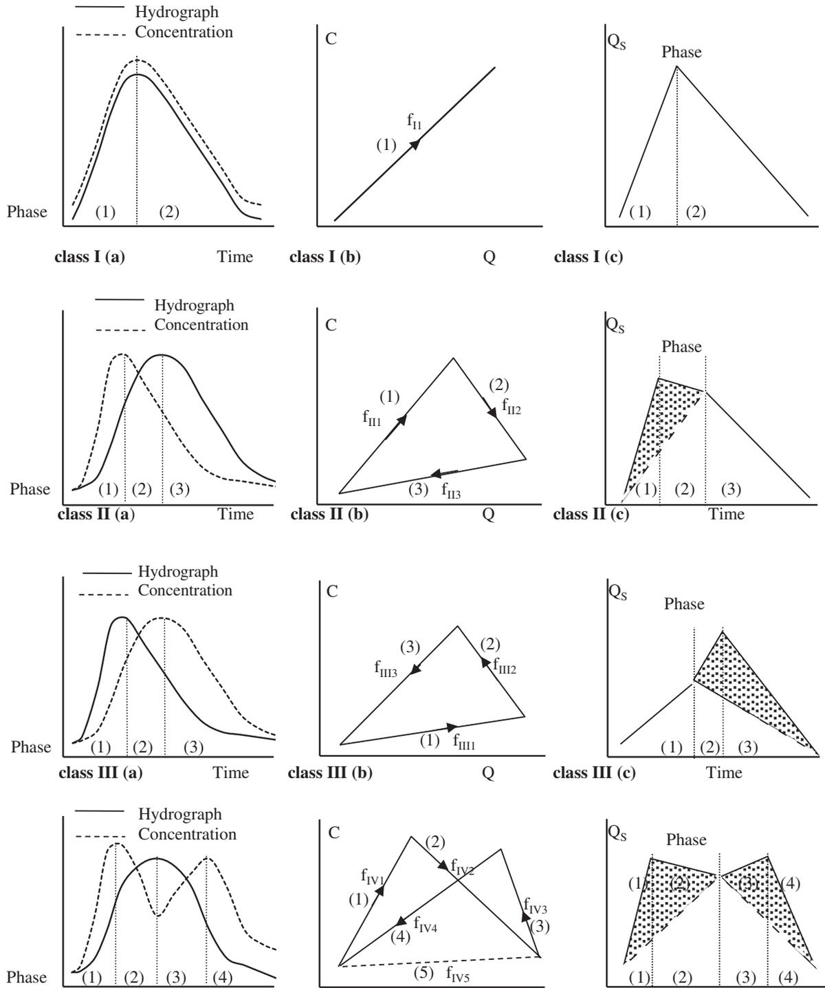
Fig. 2. Common relationships between suspended sediment concentration (C) and discharge (Q); identification of successive stages of a flood event and schematic diagram explaining evaluation of the two components: base load ( $Y_{S1}$ ) and supply of new sediment sources, available in the river basin ( $Y_{S2}$ ).
