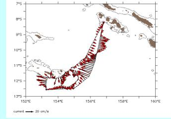
Cross track geostrophic current referenced to 700 m depth from the T S profiles
