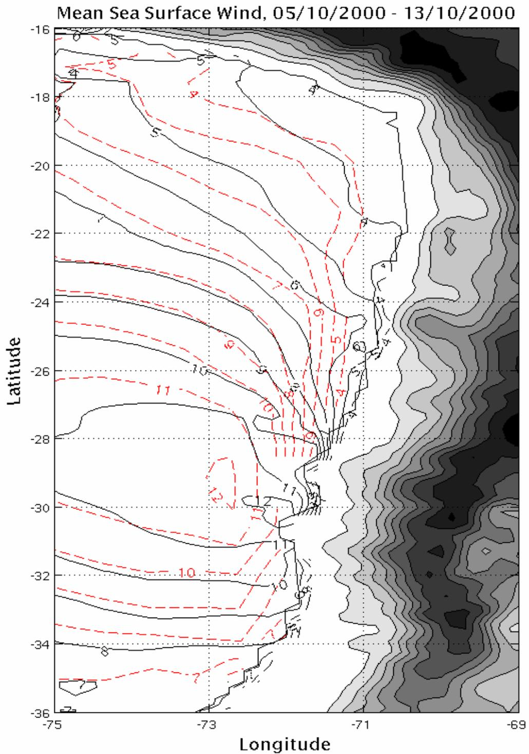
Mean Sea Surface Wind during the period 05/10/00 – 13/10/00. In red dashed-line, WRF with a 56 km resolution, in black solid line, WRF with a 18 km resolution
