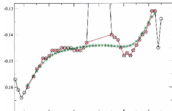
**Figure 1:** T/P wet tropospheric corrections (Track 22, Cycle 95). Black: rough corrections. Red: valid corrections. Green: corrections reconstructed using a Bezier polynomial technique.
