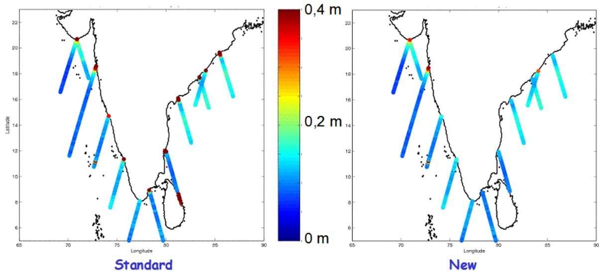
**Figure 4 :** Alongtrack standard deviation obtained (from cycle 5 to cycle 364) a) when using a standard processing and b) when using the Albicocca chain.
