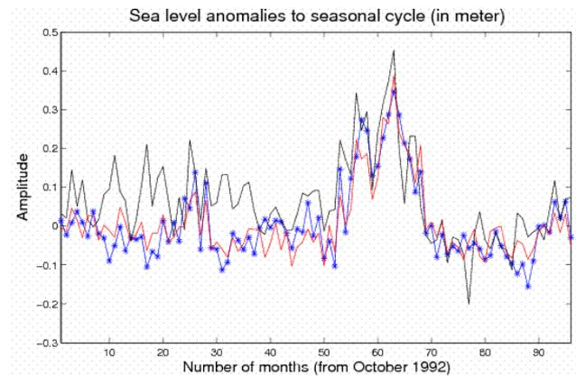
**Figure 8 :** Sea level anomalies with respect to the seasonal cycle at Lobos (6.93°S) for a) tide gauge data (blue), and for alongtrack T/P coastal data using b) a standard processing (black) and c) the the Albicocca chain (red).
