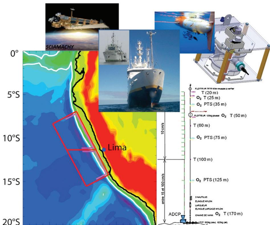
▲ Figure 1: General schematic AMOP strategy (below on the left) including in situ observations: French (red track) and Peruvian (pink track) Research Vessels, a subsurface mooring, gliders, innovative systems (e.g. *In situ* Oxygen Dynamics Autoanalyzer: IODA) as well as satellite and modeling approaches.
