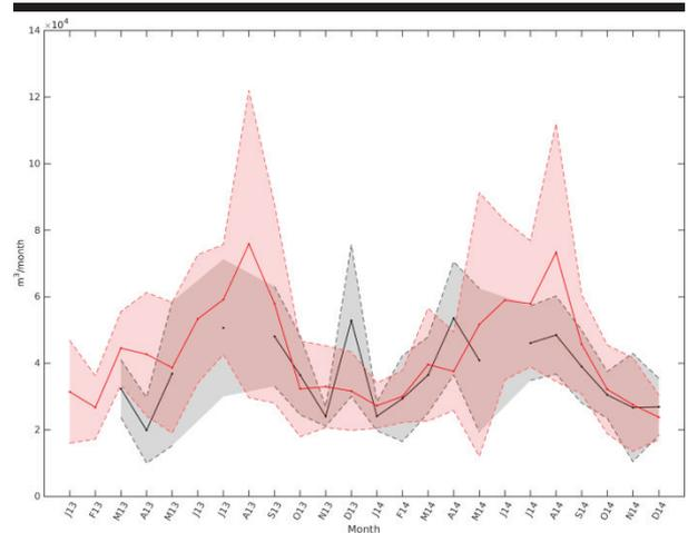
Figure 4. Monthly video estimates of Longshore Sediment Transport estimated using the Kaczmarek *et al.* (2005) formula, computed from (red) ERA-Interim re-analyses (using Larson *et al.*, (2010) for wave propagation to the shore) and (black) video estimates. Shaded zones stand for day-to-day dispersion (standard deviation).
