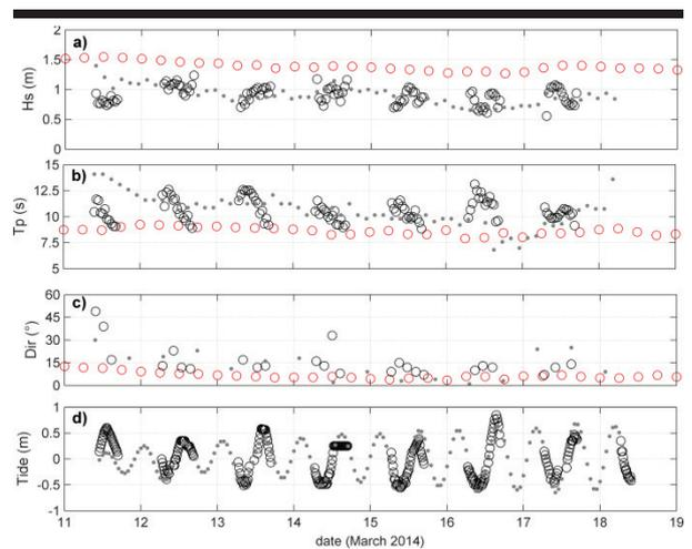
Figure 2. Comparison of 15-min video estimates with Grand Popo 2014 hourly field measurements for (a)  $H_s$ , (b)  $T_p$ , (c)  $Dir$  and (d) tide. Red circles stand for ERAInterim waves propagated to the shore using formula by Larson *et al.*, (2010). Grey dots and black circles are in-situ data (ADCP) and video data, respectively.
