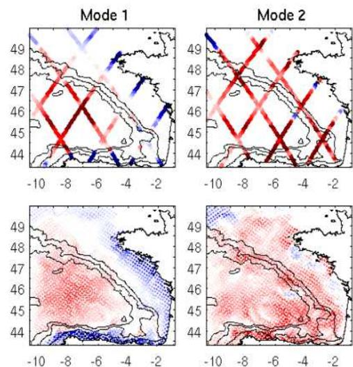
Fig2: Modes 1 and 2 for JASON (top) and SWOT (bottom). Both JASON and SWOT would be able to detect the large-scale water sloshing motion between the shelf and the abyssal plain, but only SWOT could consistently detect coastal mesoscale and high-frequency processes.
