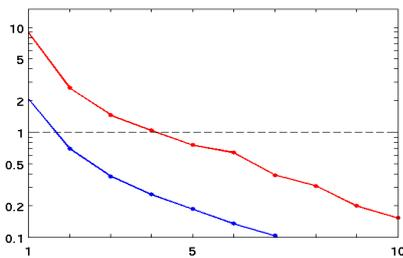
Fig1: Representer matrix eigenspectra for JASON-1 (a nadir-observing altimeter, blue) and SWOT (a wide-swath altimetry project, red). (Log scale.) The observational noise floor is shown as a dotted line. SWOT would be able to detect 4 d.o.f.s (degrees of freedom) of prior state error, while JASON would only detect 1 above the noise floor. But which error modes?
