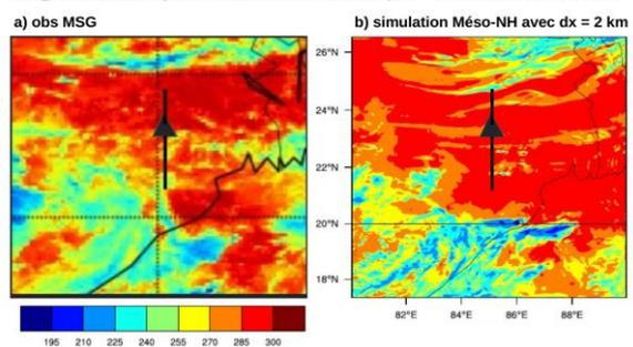
Brightness temperature at 10.8  $\mu\text{m}$  on 08 August 2017 at 0600 UTC as (a) observed by the SEVIRI imager on MSG satellite and (b) simulated with Meso-NH.
